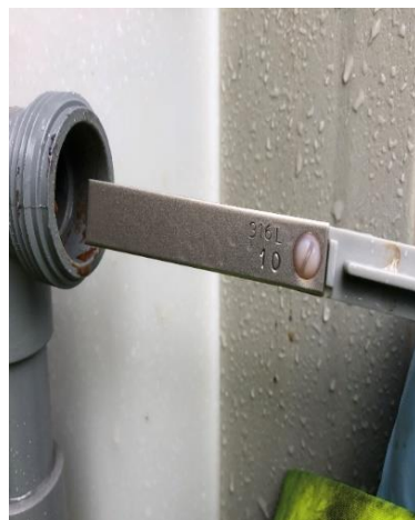
The corrosion rack assembly
